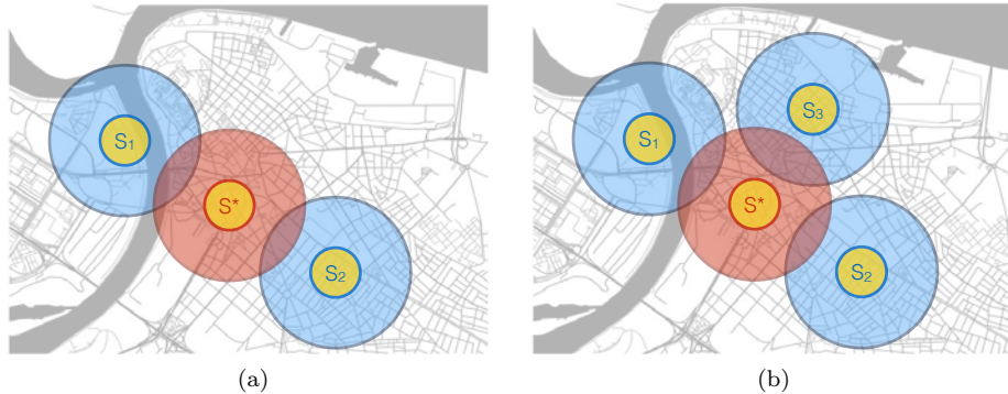
Figure 1: Sensor placement example demonstrating (non-negative and monotone) submodularity. Adding a new sensor s^* to the set A = \{s_1, s_2\} (shown in part a) is more valuable than adding it to the superset B = \{s_1, s_2, s_3\} (shown).
